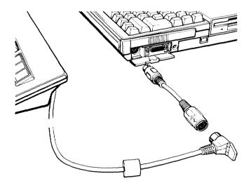
You only need the keyboard adapter if your keyboard connector interferes with the RGB VIDEO port and you are planning on connecting an external monitor to this port.
